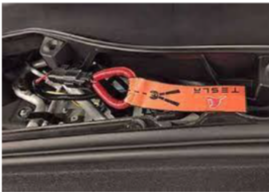
Image of a First Responder cut loop
