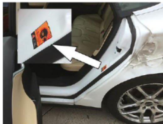
Image of a Factory Identified High Voltage Disconnect
